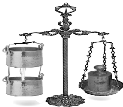
Figure 4. Galileo's installation for determining the force of impact
