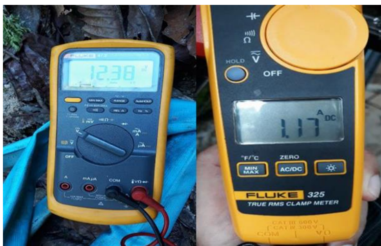
Figure 11. (a) voltage output and (b) current output of the Pelton wheel micro-hydro
