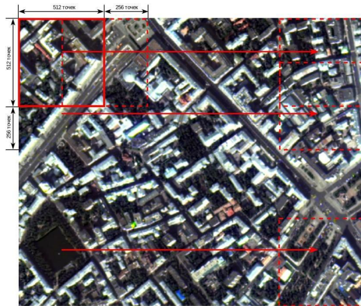
Figure 03. Splitting the original image into pieces of fixed size, using the sliding window method.
