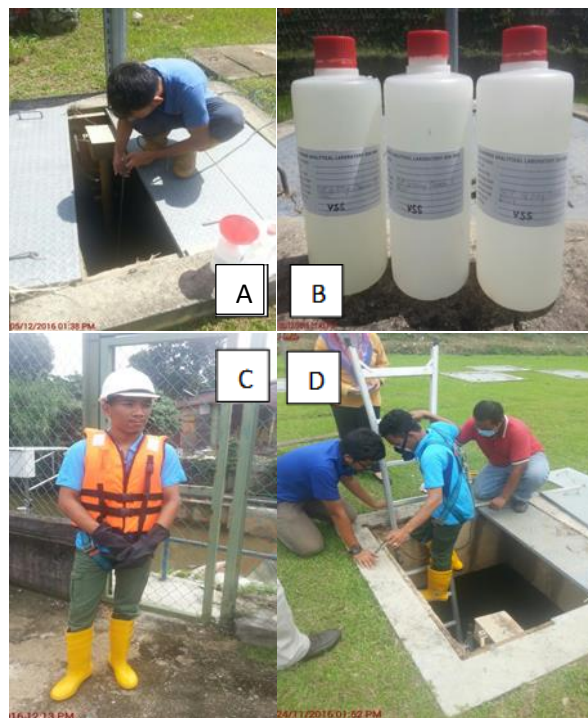
Figure 04. (A) Sampling work for MLVSS Sample (B) MLVSS Sampling Bottle (C) Safety Outfit for TVS Sampling (D) TVS Sampling work in RWTP oxidation chamber
