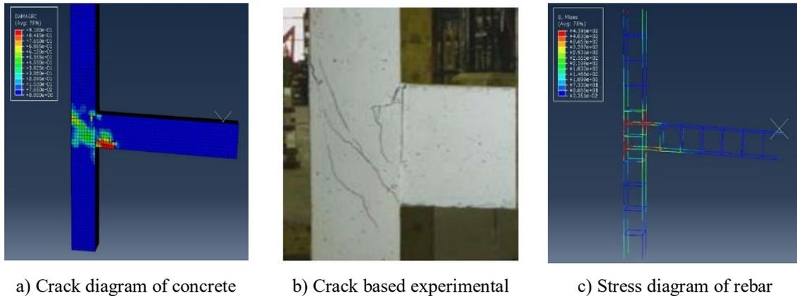
**Figure 05.** Comparative analysis of the experimental test and numerical analysis at the maximum loading
