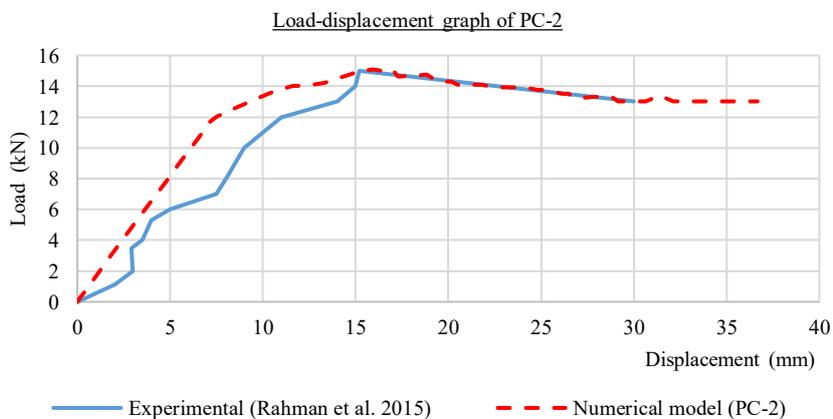
**Figure 07.** Comparison results of experimental results and numerical results (PC-2)
