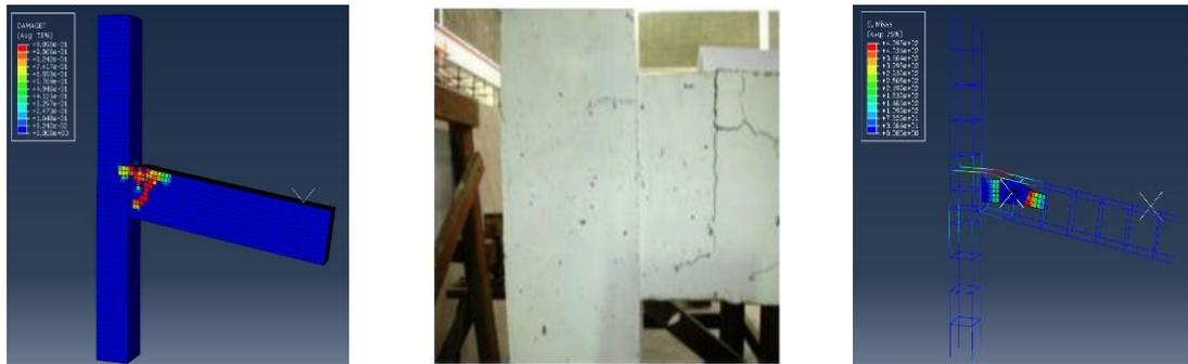
a) Crack diagram of concrete
