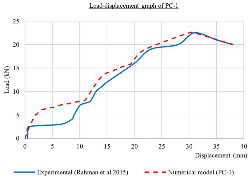
**Figure 04.** Comparison results of experimental results and numerical results (PC-1)
