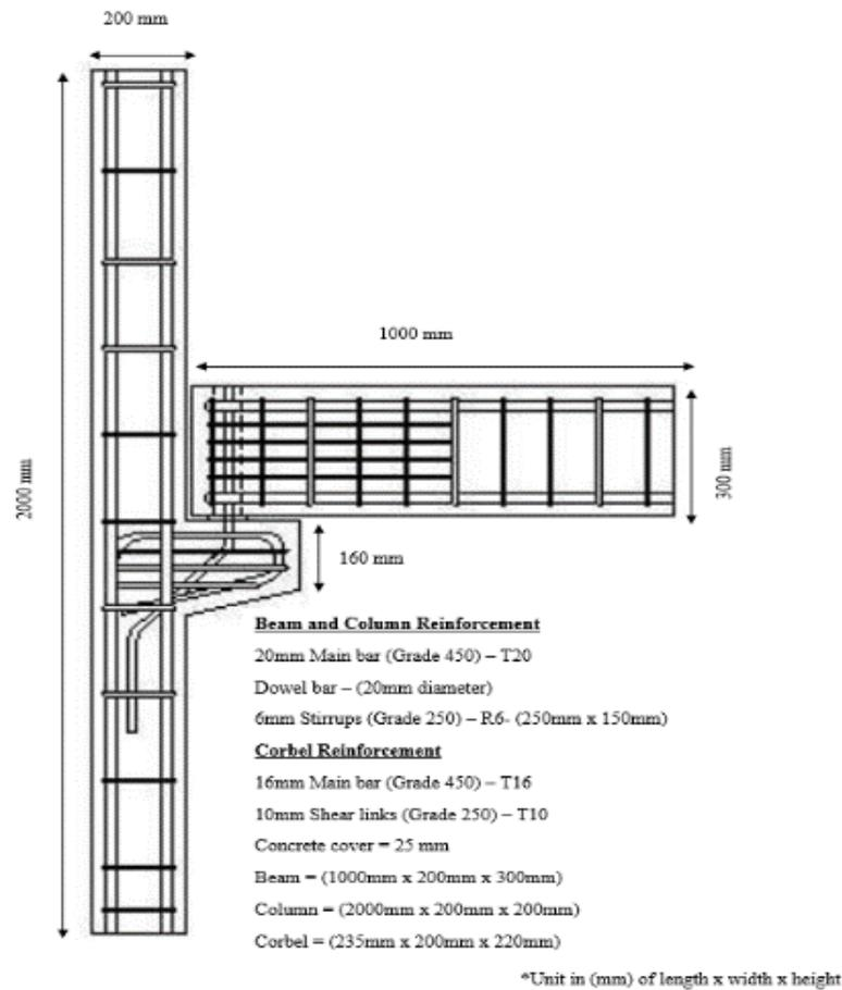
**Figure 02.** Type precast beam to column connection model Source: Modified from Rahman and Leong (2006)
