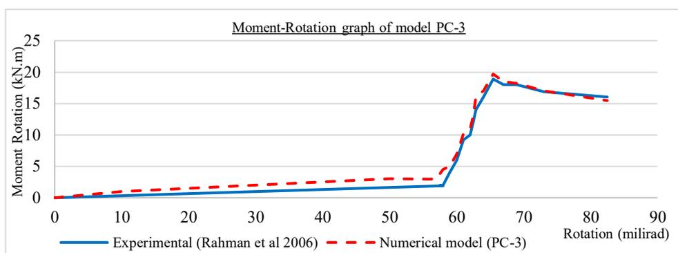
**Figure 09.** Comparison results of experimental results and numerical results (PC-3)
