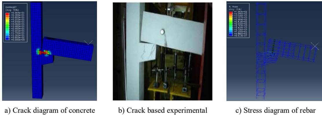
**Figure 10.** Comparative analysis of the experimental test and numerical analysis at the maximum loading
