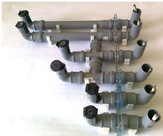
Figure 02. Two-chamber membrane type MFC
