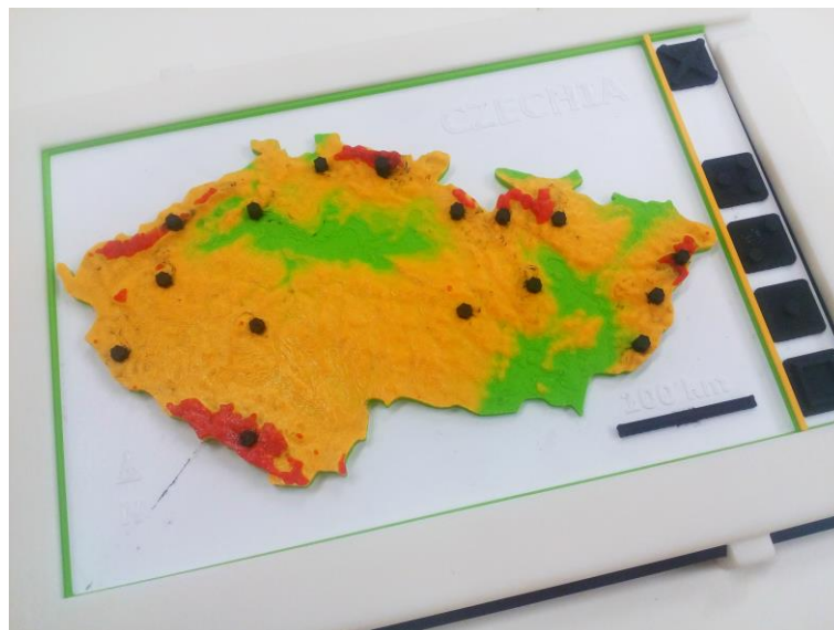
Figure 04. An altitude map of the Czech Republic (Czechia), using TouchIt3D technology. TouchIt3D tactile maps use special software (TactileMapTalk) that is installed on the tablet.
