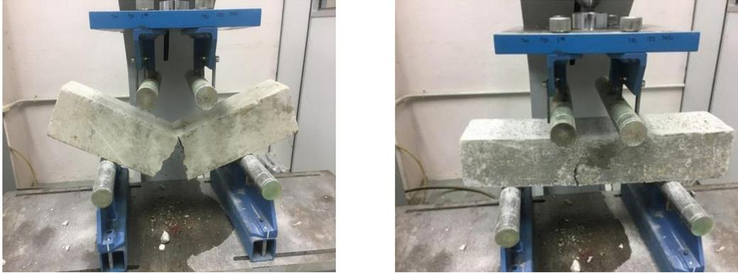
**Figure 04.** Crack pattern without (left) and with (right) steel fibres
