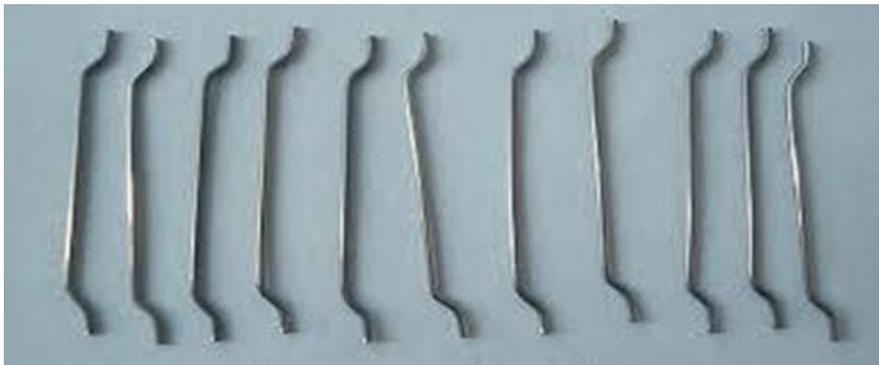
**Figure 01.** Steel Fibres
