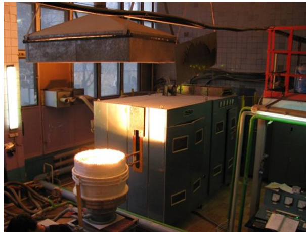
Figure 02. Installation of high power with a crucible diameter of 700 mm during the synthesis of PSZ crystals
