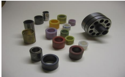
Figure 05. General view of the bearing bushings from PSZ used in the submersible pump section
