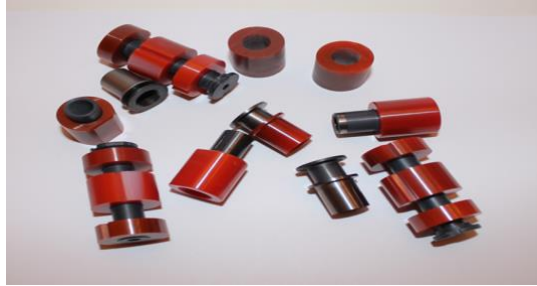
Figure 04. Journal bearing bushings made of PSZ crystals
